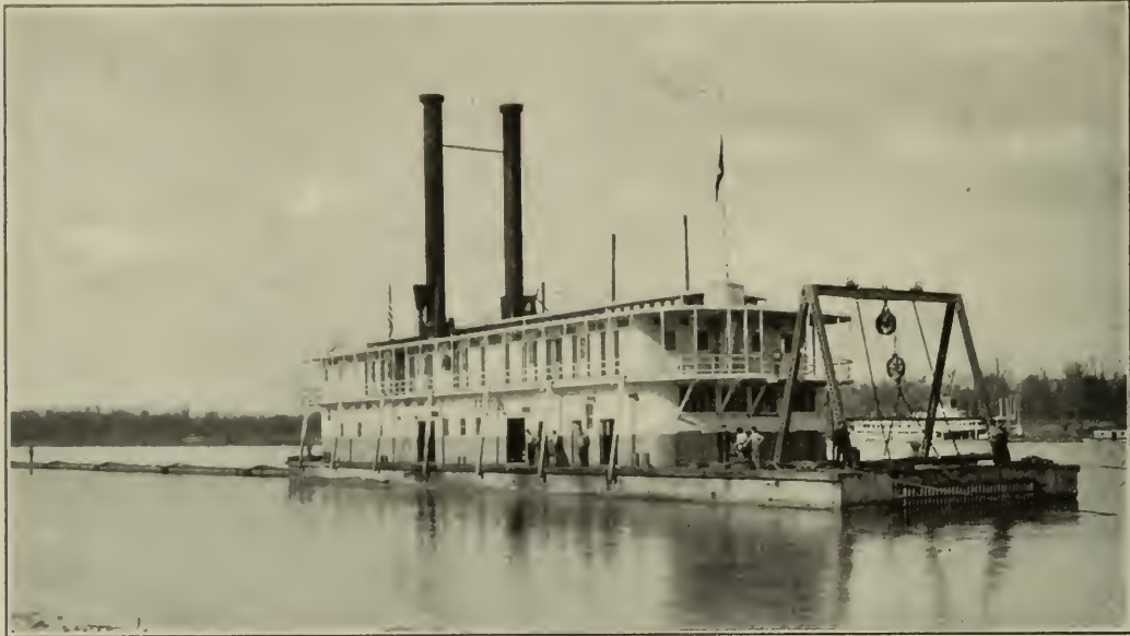
FIG. 29. HYDRAULIC DREDGE EPSILON, MISSISSIPPI RIVER.
